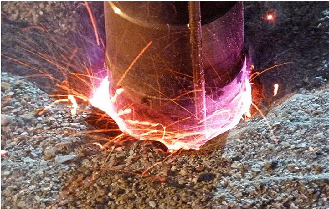
Figure 4: GA Drilling's PLASMABIT in action (GA Drilling official website).
