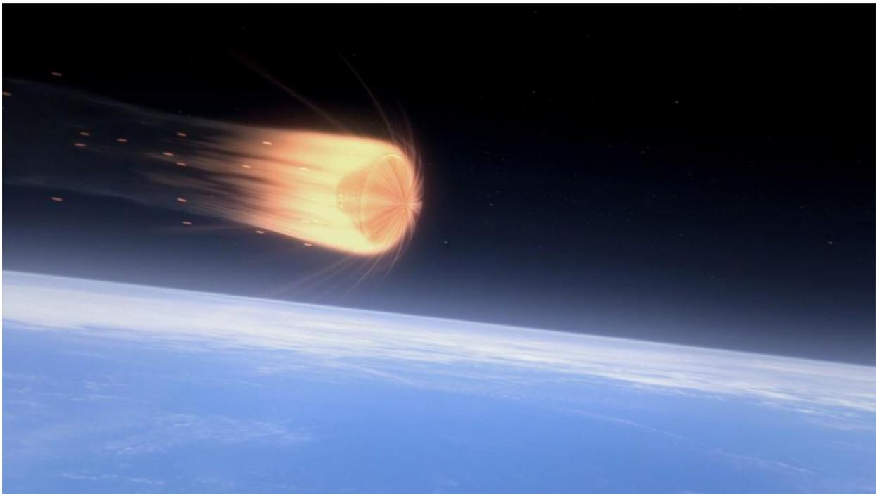
Figure 32: Orion with its base heat shield facing Earth as it encounters the first areas of the discernable atmosphere around the planet and the temperature around the spacecraft begins to build up (Siceloff).
