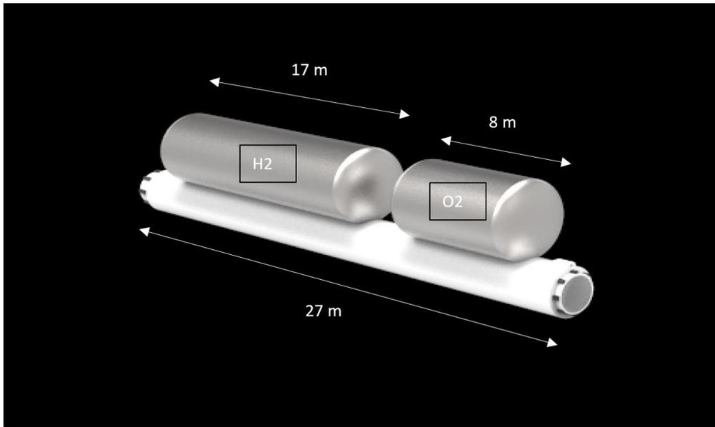
**Figure 4.2.2c.** Module 2 (oxygen and hydrogen tanks) of refueling depot.
