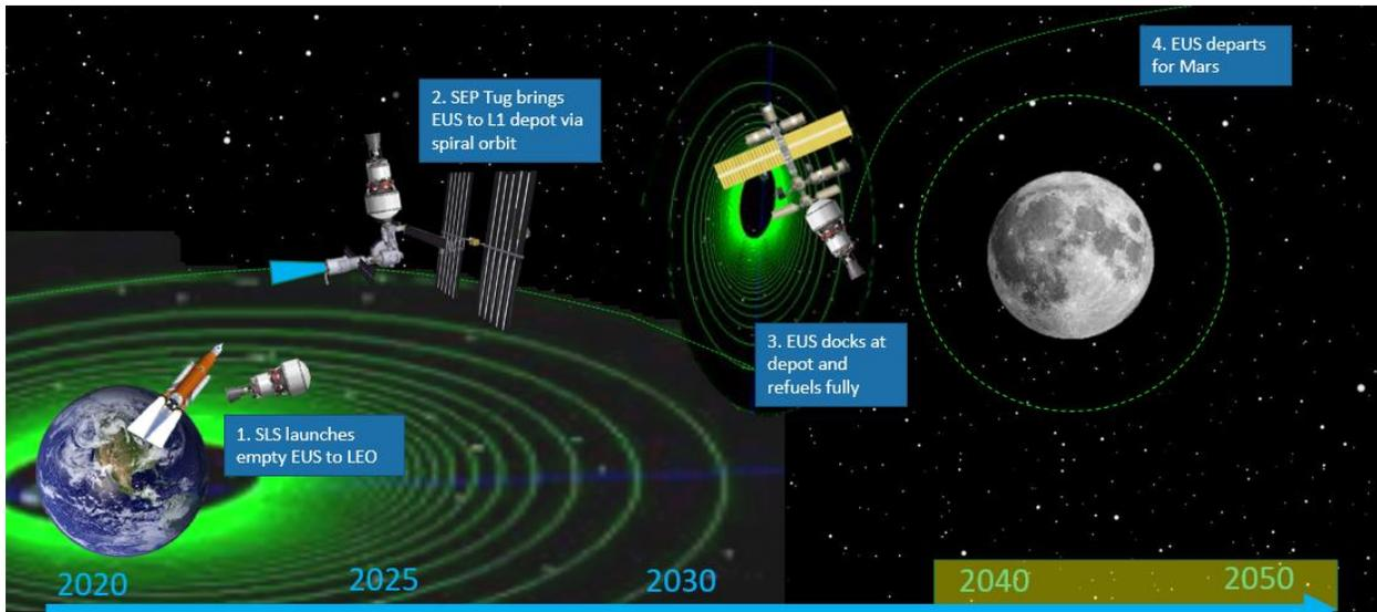
**Figure 6.3b.** The schematic above describes the tug-assisted timeline operations once the fully operational phase is reached in the 2040s.
