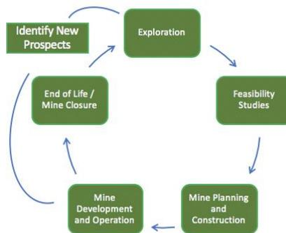
**Figure 3a.** *Typical Mining Life Cycle.*
