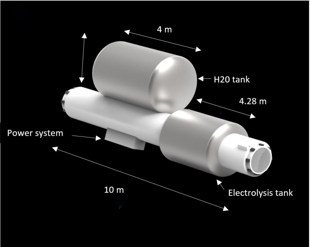
**Figure 4.2.2f.** *Module 4: electrolysis extension module.*
