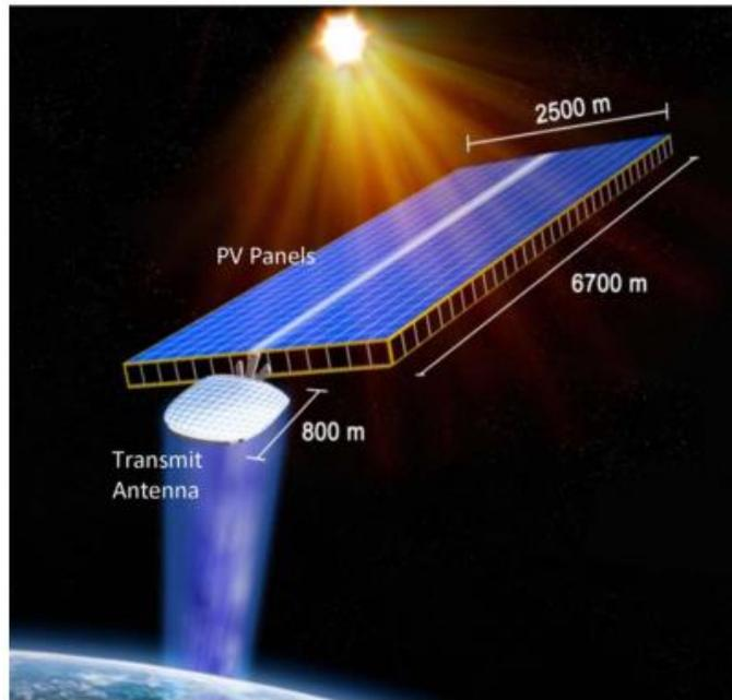
**Figure 4.1.5a.** *Illustration of microwave energy transmission.*
