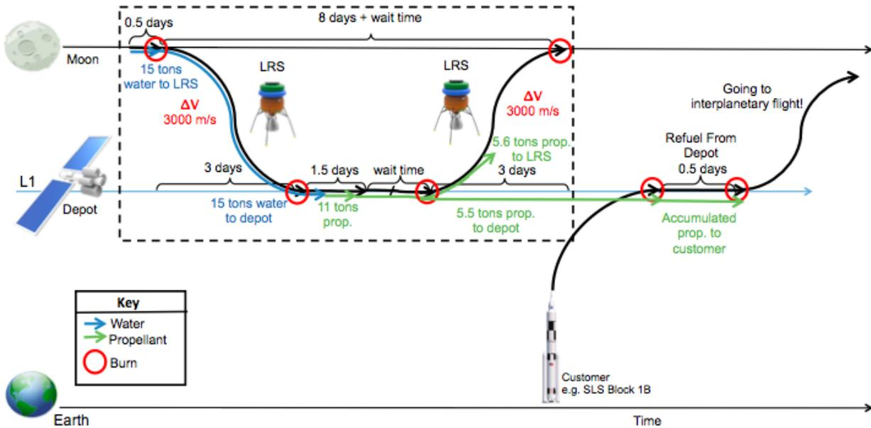
**Figure 4.2.1a.** The LRS flies cycles between the Depot and the Base to transport water. After the cycle in the dashed box is repeated several times, enough propellant is deposited at the Depot to support a customer mission.
