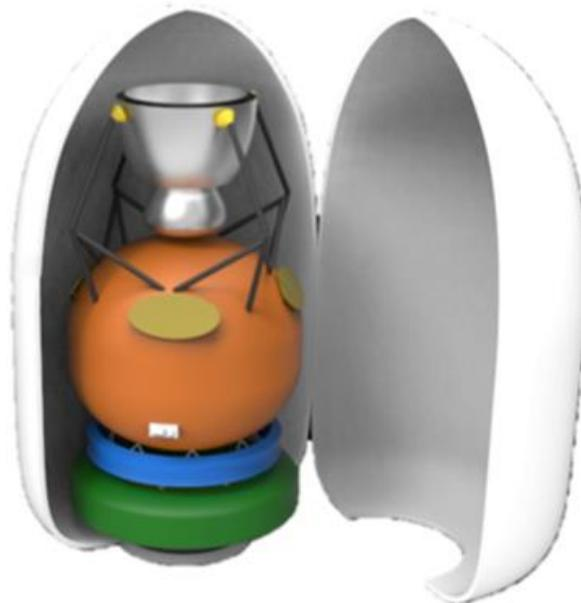
**Figure 4.2.1d.** Stowed configuration of the LRS.
