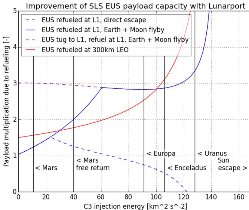
**Figure 5.3b.** A threefold increase in the payload capacity of the Space Launch System’s (SLS) Exploration Upper Stage (EUS) to many destinations can be achieved by using Lunarport.
