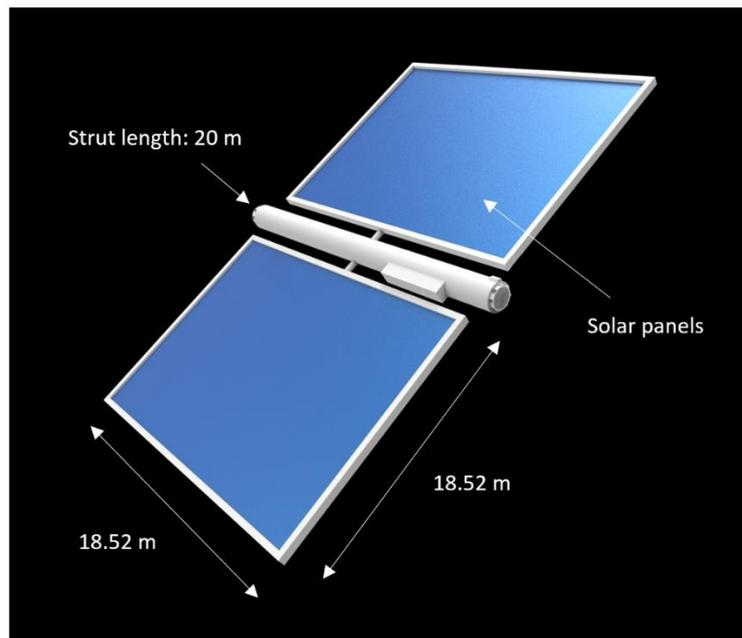
**Figure 4.2.2d.** Module 3: solar panel extension module.
