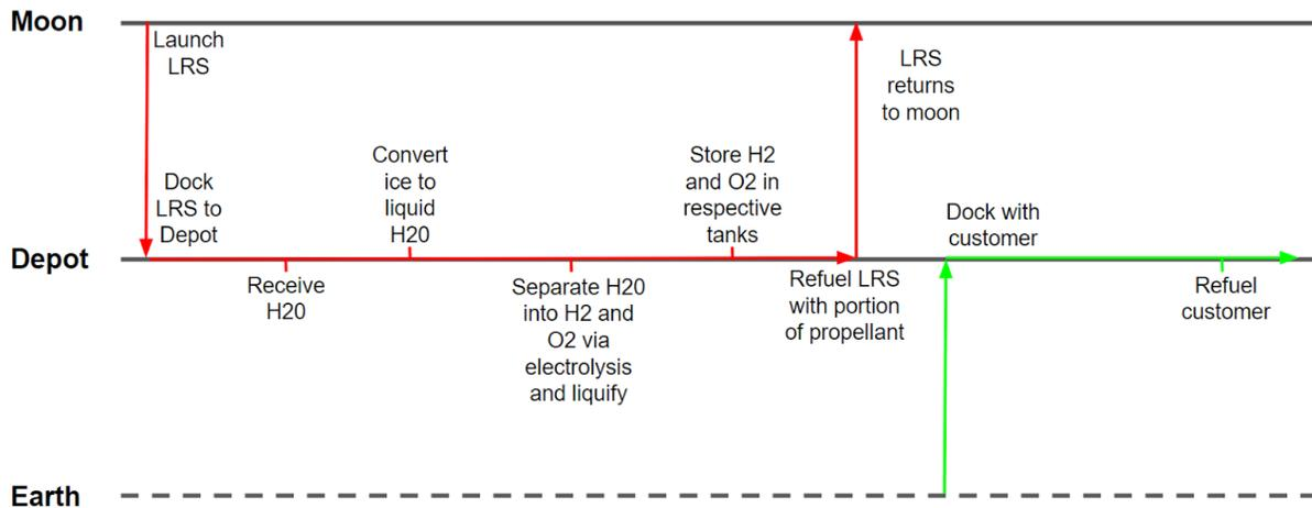
**Figure 4.2.2a.** Concept of Operations for the refueling depot.
