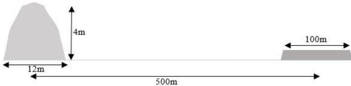
Figure 4.1.6c. Covering berm Diagram.
