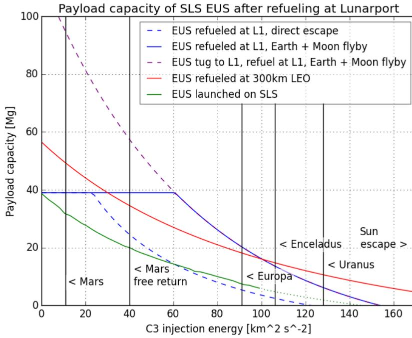
**Figure 5.3a.** Refueling at Lunarport’s L1 depot increases the payload capacity of the Space Launch System’s (SLS) Exploration Upper Stage (EUS).
