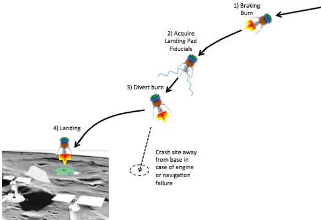
**Figure 4.2.1b.** *The descent trajectory of the LRS is designed to reduce the risk to Base infrastructure in the event of an LRS failure.*
