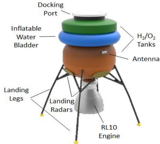
**Figure 4.2.1c.** Configuration of the LRS with key parts labeled.
