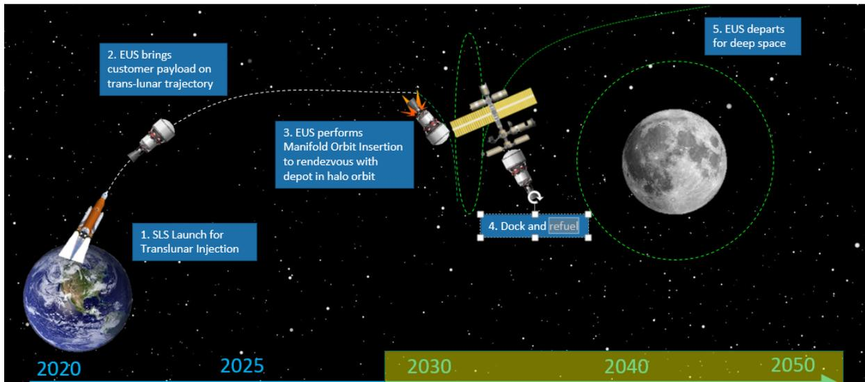
**Figure 6.3a.** The operational phase above is reached when the depot begins reaching 120 t capacity with the required delivery cadence from the LRS.
