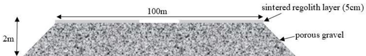
**Figure 4.1.6b.** Launch Pad Construction.
