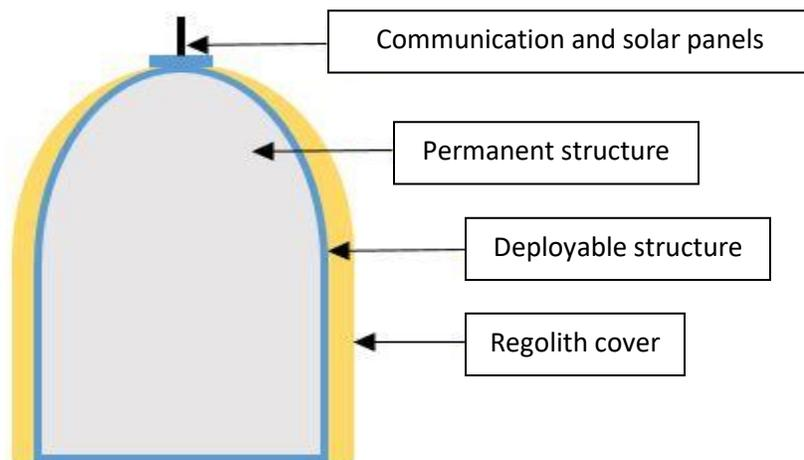
**Figure 4.1.8a.** *Regolith protection structure schematic.*
