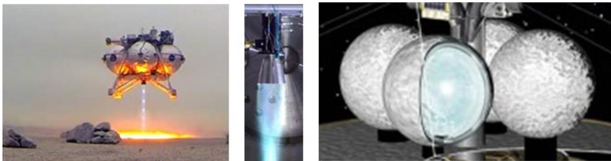
**Figure 4.2.1e.** Technologies needed for the LRS are already under active development. JPL's ALHAT sensor demonstrates using terrain-relative navigation for precision landing (shown on left, in a test flight on the Morpheus lander). ULA is test-firing H<sub>2</sub>/O<sub>2</sub> reaction control thrusters for their Advanced Cryogenic Evolved Stage (middle). TransAstra is developing flexible water bladders under a SBIR contract (right).
