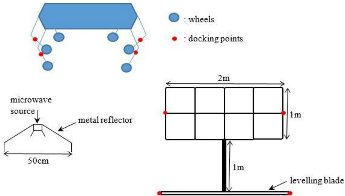
Figure 4.1.1a. Sintering robot diagram.
