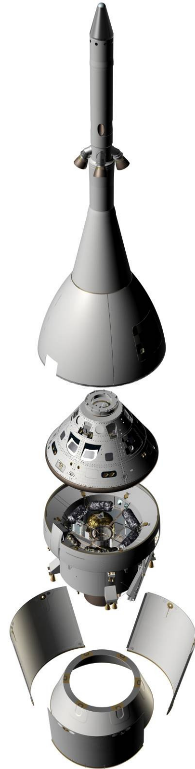
Figure 4: The Orion Spacecraft. From top, Launch Abort System, Crew Module, Service Module, Spacecraft Adapter.
